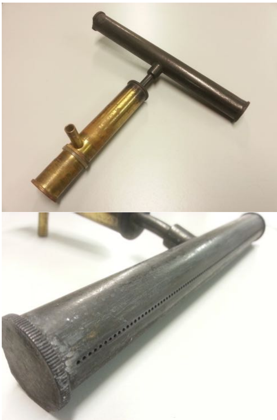
Figure 5: Smoking burner at Adelaide, made by Palmer (London). There are three of these: this one 22 cm wide, and two others 15 cm wide. The holes of all three are 1 mm in diameter, centres spaced 2 mm apart. The lower end has a capsule for benzol.
