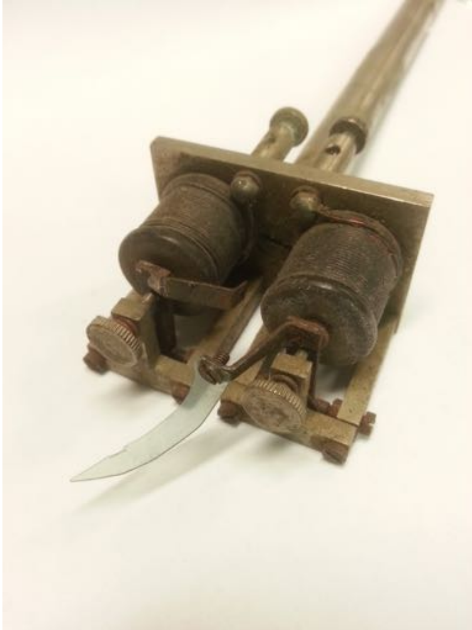
Figure 3: A signal writer with a plastic writing-point, University of Adelaide Heritage Collections. A current through the electromagnet moves the lever. This particular signal writer has two independent electromagnets, allowing two independent traces.
