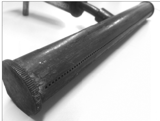
Figure 4: Smoking burner at Adelaide, made by Palmer (London). There are three of these in the Adelaide Heritage Collections: this one 22 cm wide, and two others 15 cm wide. The holes of all three are 1 mm in diameter, centres spaced 2 mm apart. The lower end is a capsule for benzol.
