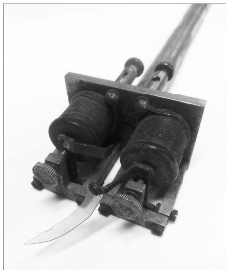
Figure 2: A signal writer with a plastic writing-point, University of Adelaide Heritage Collections. A current through the electromagnet moves the lever. This particular signal writer has two independent electromagnets, allowing two independent traces.
